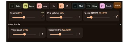
The **Master** section allows you to adjust the signal output levels. Available parameters:
